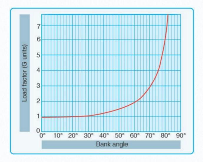
This task is pretty simple. Just find the bank angle on one axis, trace it to the line, and find the load factor on the other axis.
