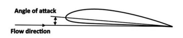
An aircraft's wings or rotors don't cut through the air like a knife, they are angled slightly upwards. This way, the wind hits the bottom of the wing and pushes the aircraft from below. It also creates lift from above (check out Bernoulli's principle here if you're interested in the physics).
